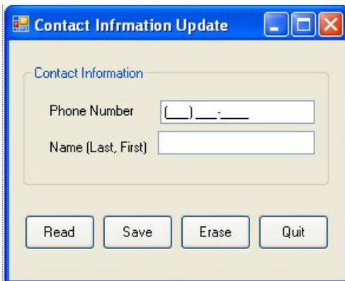
In this application, existing contact data are read from an existing file when the Read button is clicked. Whatever contact information on the screen will be saved onto another file when the Save button is clicked. An open file dialog and a save file dialog are used to prompt for the file paths.
